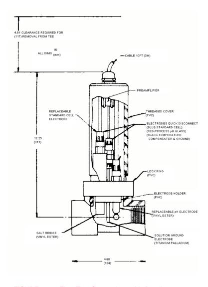
FIGURE 27-1: Flow-Thru Sensor Assembly Details
