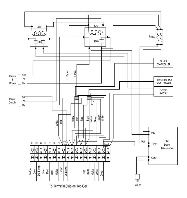
FIGURE 9-12: Wiring Diagram
