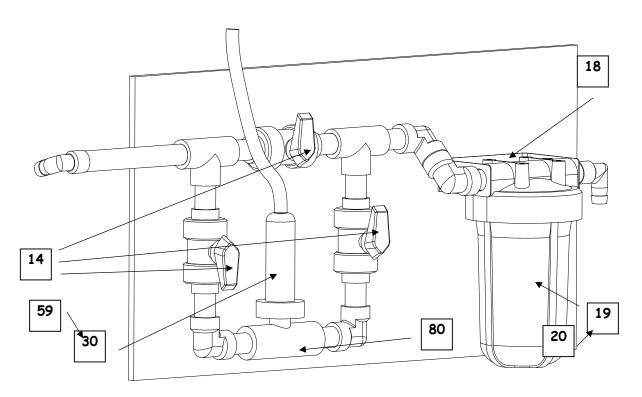
FIGURE 9-4: Silver Probe with Filter Chamber
