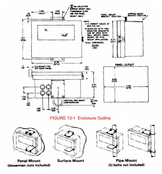
FIGURE 13-2 Mounting Configurations
