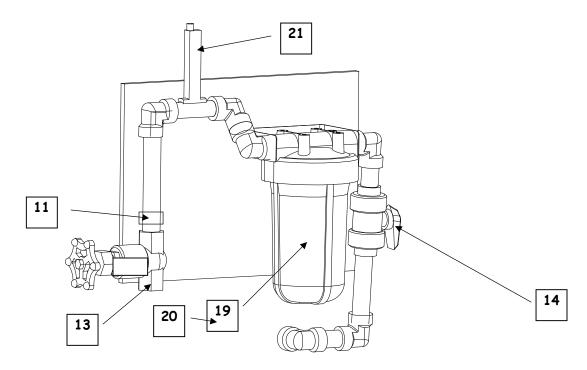
FIGURE 9-3: Flowmeter with Filter Chamber
